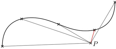
Fig. 1. Distance computation. Several points are sampled uniformly on the curve. The distance of a data point  $P$  to the curve is approximated by the distance to the closest sample point (red line).
