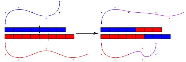
Fig. 2. One-point crossover. The parents are cut after position 4 and 5. Blue and red curve segments are influenced by control points of one parent. Purple curve segments are influenced by control points of both parents.
